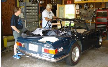
New tops usually come with a bag of loose snaps that need to be placed in the proper locations.
