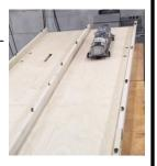
front of the racer doesn't hit the ground when leaving the track, and the rear doesn't drag on the track when it completely exits, you can't have too much car protruding at the front or back relative to the wheels. Thank you to Larry Berg and Joe
